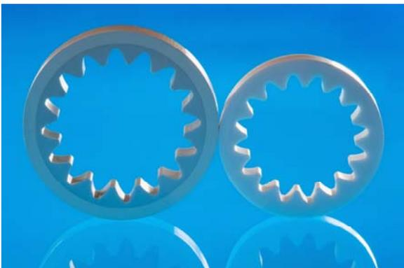
Fig. 5 Ceramic gear wheel in the green and sintered state made by two-component CIM combining alumina and zirconia toughened alumina (source: Fraunhofer IKTS, Designed by Robert Bosch GmbH)
