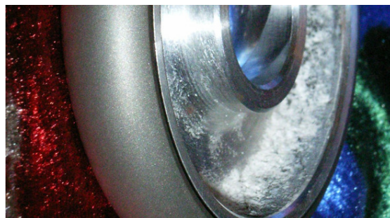
Fig. 2: conTEX still clean after 6 months production of 6 different spun dyed yarns without cleaning.
